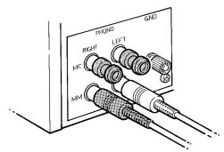
The other set of jacks is marked MM, for Moving Magnet. If you have a regular moving magnet cartridge mounted on your turntable, connect the turntable only to the MM inputs, as the sizeable volume boost of the MC jacks will cause volume problems and severe distortion.
